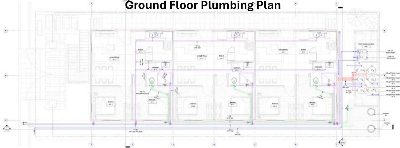
1 Ground Floor Plumbing Plan (Floor Routing) 1 : 42
